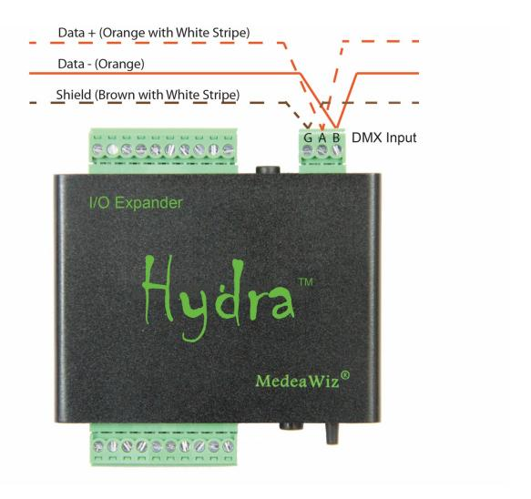
The DMX Port should only be connected to a DMX 485 bus device. Standard A, B and Ground / Shield terminals are provided. Commonly used colors are shown for Cat 5 cable above. Your colors may vary. DMX wiring for XLR and RJ45 connectors are shown below.
