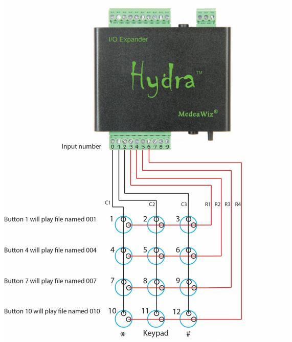
Keypads vary by manufacturer. The Columns and Rows may be in a different order than shown.
