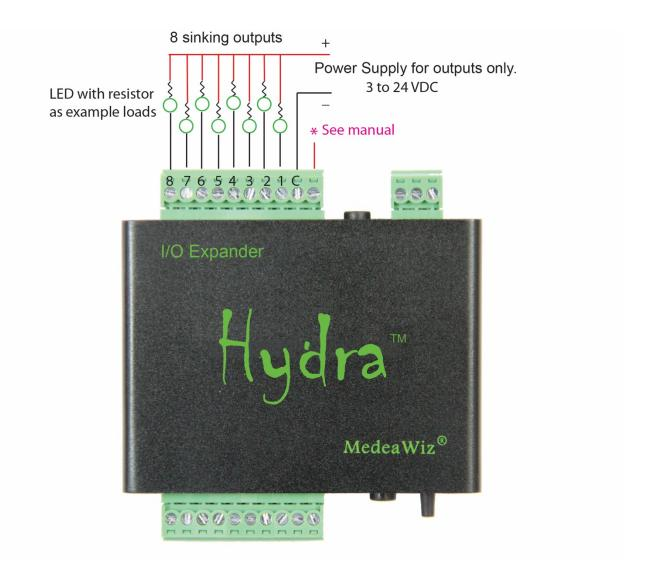
The Hydra has "sinking outputs", which means that it switches the Ground or "Minus" side of the power supply. In this case you will connect the Positive "Plus" of your external power supply directly to all output devices. The Negative "Minus" side of each output device will connect to one of the output numbers 1 through 8 on the Hydra.
