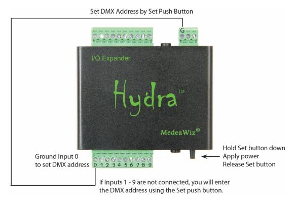
Please refer to Setting Mode by Push Button on page 21. The procedure to set the DMX address by push button is the same.
