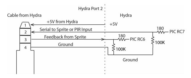
The Hydra Port 2 can be used for a second Sprite or as an input for a motion sensor or other trigger. The use depends on the operation Mode that you select from the table on page 4.
