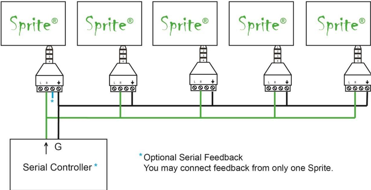
Limitations on the number of Sprites on the bus include length of wire, type of wire and baud rate. Low capacitance wire and lower baud rates will allow longer distances and / or more Sprites on the bus.
