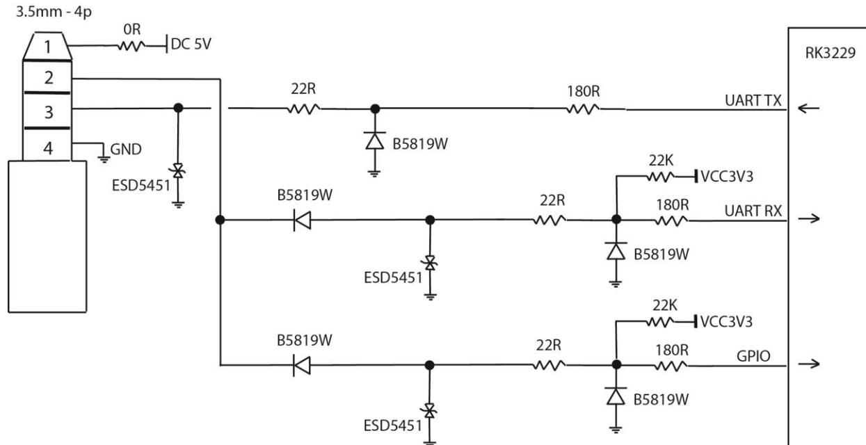
The Sprite is designed to work with serial data at 3 to 5 Volt TTL levels.
