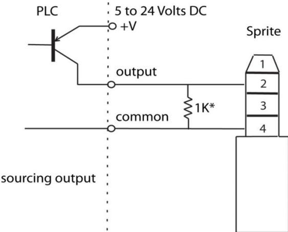
The Sprite® 4K has an internal 22K pullup so the Sourcing output requires a low resistance from Output to Common to pull the Sprite’s internal voltage down to a “LOW”. The 1K\* shown is an example and can vary depending on the +V voltage. Consider the Watt rating of the resistor.
