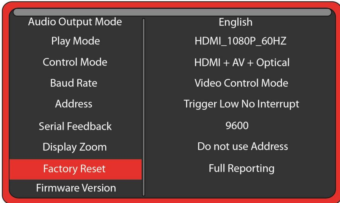
Select Factory Reset and press the green Enter key on the remote control. Then when the pop-up window appears, select “Yes” and press “Enter” to reset the Sprite® to the factory settings.
