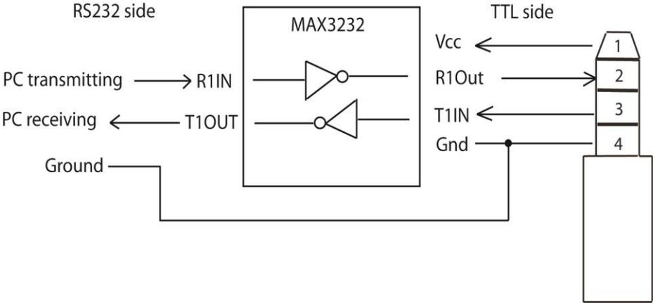
The MAX3232 can be powered from the Sprite® 4K. Connect all Grounds together.
