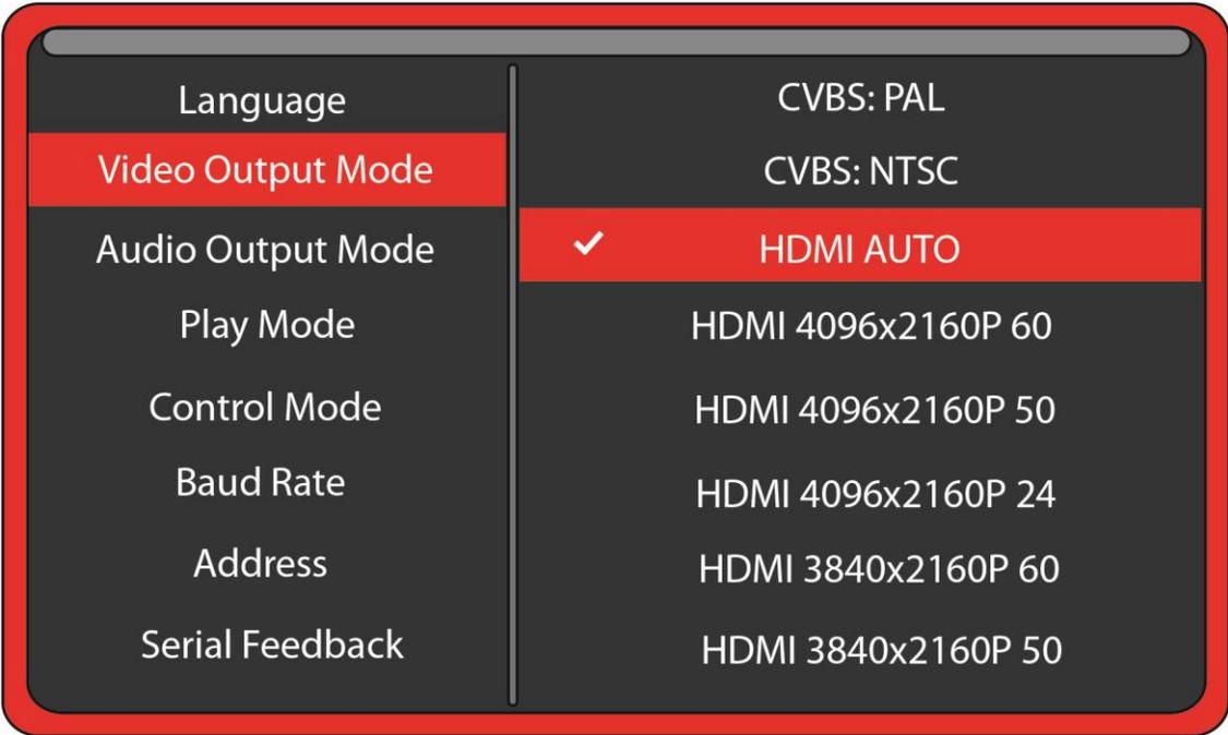
Select **NTSC** to use the Composite video output from the 3.5 mm yellow AV jack. Use the yellow RCA plug from the included AV cable.
