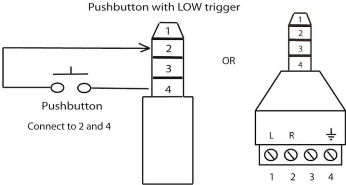
The Control Mode should be set to Trigger Low No Interrupt or Trigger Low with Interrupt or Trigger Low Delayed.
