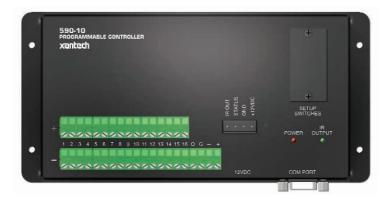
The 590-10 gives the custom installer the ability to use any push button or contact closure to initiate infrared commands. The 590-10 incorporates 16 isolated input circuits and a learning microprocessor. There are 16 pairs of screw terminals on its rear panel for use with up to 16 individual contact closures.
