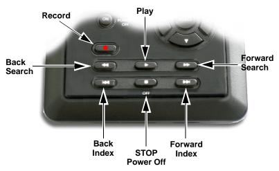
Use these buttons to control FS-4 HD playback and record functions. You usually operate these transport buttons while on the **HOME** Screen.
