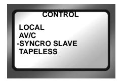
The Control screen provides the capability of enabling the FS-4 HD to operate in four different control modes during record and playback.
