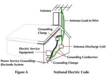
If an outside antenna or cable system is connected to the FS-4 HD/Pro HD, verify that the antenna or cable system is grounded. This provides some protection against voltage surges and builtup static charges.
