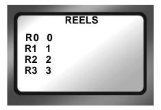
When a disk is formatted, the FS-4Pro HD creates 10 folders, numbered 0-9, on the disk. During recording or playback of a clip, it is possible to place it into folders or play it from up to 10 different reels.
