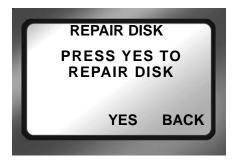
Use this function if a recording session does not complete properly and there is a question that the file may be damaged. For example, recording terminates due to a loss of power to the FS-4 HD. Repair Disk scans the entire disk drive checking for and repairing file errors and incomplete files. When the file is repaired it is can be used in the NLE system.
