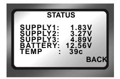
The FS-4 HD Status screen provides details of the systems power state as well as internal temperature. This screen may assist Focus Enhancements Technical Support in determining power and thermal problems with your unit.
