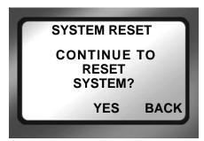
The System Reset feature restores the factory default settings for the FS-4 HD unit. This feature is useful for diagnosing problems with the unit.
