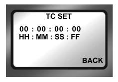
The Timecode Set parameter stores a user defined timecode in the FS-4Pro HD's non-volatile memory. This value is available for use by the FS-4Pro HD immediately after exiting **TC SET**.
