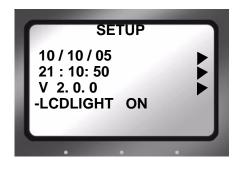
The items on the Setup Screen are grouped by function. Within the function the items act like radio buttons, i.e. when one is active the others are not.
