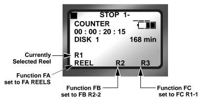
The function buttons are a quick way to mark video clips during recording. The Functions menu offers two types of markers to use, as an example **FA REELS** and **FB R2-2**.
