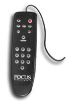
When using the optional wired remote control, use the button pad numbered 0-9 to mark the clips. Any additional button presses during a recording or playback, changes the selected REEL. Once a session is finished, select **Organize REEL** in **Utilities** screen. The marked clips are placed in the REEL folders in sequential order.
