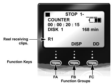
Function settings are user-assignable and available in the Functions screen. Changing a setting with a Function button has the same effect as manually changing the setting.
