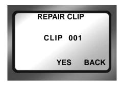
Use this function to repair a specific file that may be damaged or incomplete. For example, recording terminates due to a loss of power to the FS-4 HD and a specific file may be damaged. Repair Clip scans the specified file checking for and repairing file errors and incomplete files. When the file is repaired it is can be used in the NLE system.
