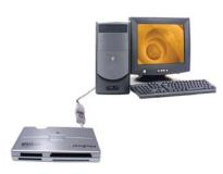
Connect your card reader to your PC (note: be sure that the card reader driver is installed) and insert the Compact FLASH card (we recommend 128 MB minimum) into the reader. To program your multimedia content on to the media card, open the file manager and copy the files to the card reader drive.
