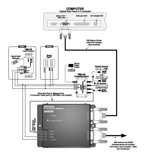
Figure 1 – Typical System Configuration with Programming Hardware Connections
