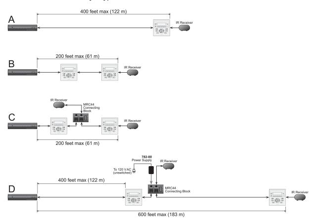
Figure 11 - MRC44 Keypad CAT5 Cable Lengths
