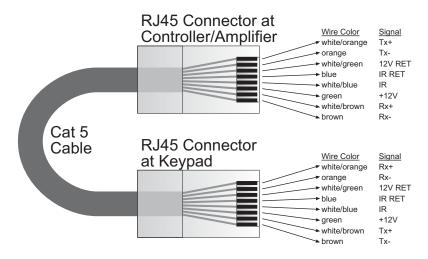
Figure 10 - CAT5 Pin Assignments (per EIA/TIA 568B)
