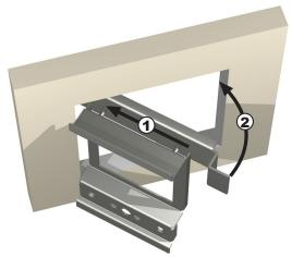
Figure 8 – Installing the MRC44 Keypad mounting bracket in the wall
