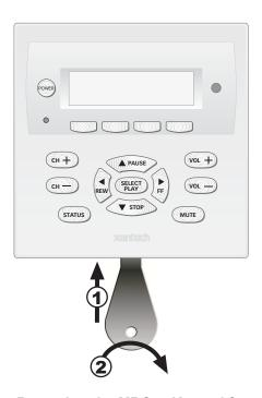
Figure 9 – Removing the MRC44 Keypad from the wall
