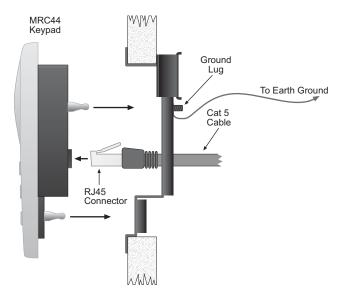
Figure 6 - Mounting and Installing the MRC44 Keypad
