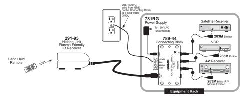
Figure 4 - Addition of System GND Wire for RF Interference Reduction
