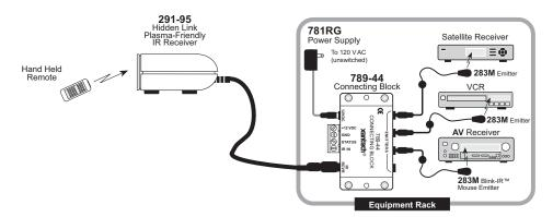
Figure 2 - Typical System Layout using 291-95, 789-44, 781RG, and 283M Emitters
