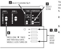
You can set up a zone to be "unaffected" when a certain scene is selected. (The unaffected zone's light levels remain unchanged when the new specified scene is selected.)
