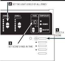
The S and M indicators under the FADE window show whether FADE is "M"inutes or "S"econds. To set FADE in minutes, you press FADE ▲ to scroll through 1—59 seconds...the M lights. FADE is now expressed in minutes. To get back to seconds, press FADE ▼ until the window shows "S"econds.
