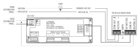
EACH TERMINAL CAN ACCEPT UP TO (2) 2.5 mm² WIRES
