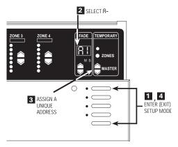
Assign each *GRAFIK Integrale* Control Unit in your project a unique system address (RI through RB).
