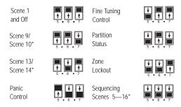
When using an Accessory Control to access scenes 5—16, the scene LEDs will illuminate only on the Accessory Control—not on the GRAFIK Integrale Control Unit.
