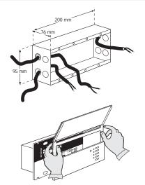
Remove Cover. Remove the Control Unit's cover and hinged faceplate by pulling outward at each corner.
