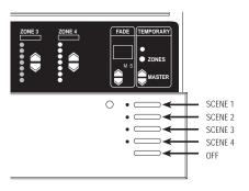
Scenes are the preset light levels and fade times stored in the Control Unit. To create a scene, set the appropriate intensity for each ZONE. To recall a scene, simply press one of the buttons. The first button calls up Scene 1; the second, Scene 2; and so on. The last button turns lights Off.
