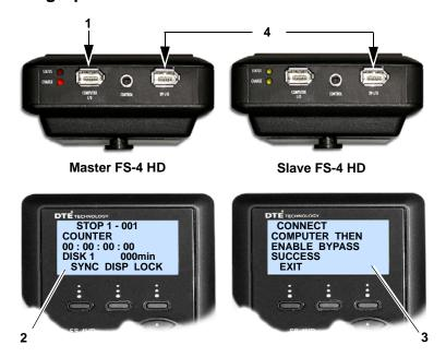
1. Connect the camcorder to the master FS-4 HD, **DV I/O** connector using the supplied FireWire cable.
