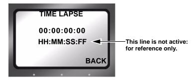
Time Lapse provides the ability to record a single frame at specific time intervals, for example one frame per minute, 00:01:00:00. Time Lapse applications can include capturing the traffic on city streets, the growth of a plant from seed to maturity, and construction projects.
