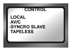
The Control screen provides the capability of enabling the FS-4 HD to operate in four different control modes during record and playback.
