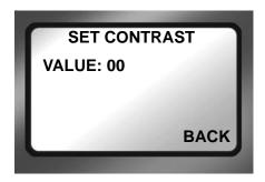
Use this function to adjust the contrast of the LCD display for easier viewing.
