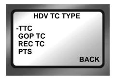
This menu sets the source of the timecode displayed in the TC DISP mode, while in HD RECORDER mode. This is also the timecode reported in AV/C control mode.
