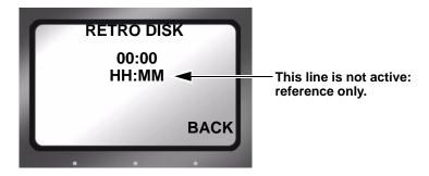
The Retro Disk mode records video in a continuous loop to a user-defined portion of disk space. Pressing Record ● seamlessly begins active recording. The Retro Disk session is appended to the beginning of the new clip. The result is a set of clips beginning with the cached video and continuing with the newly recorded video.
