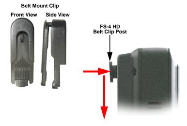
A belt mount clip is included with the FS-4 HD. This mount is similar to those used with cellular telephones. Attach the belt mount to the belt clip post on the rear of the FS-4 HD and push it down to lock it in position.
