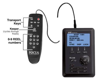
Transport keys have the same functions as on the FS-4 HD.  Use the Keeper
