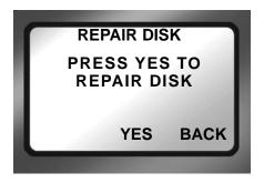
Use this function if a recording session does not complete properly and there is a question that the file may be damaged. For example, recording terminates due to a loss of power to the FS-4 HD. Repair Disk scans the entire disk drive checking for and repairing file errors and incomplete files. When the file is repaired it is can be used in the NLE system.
