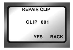
Use this function to repair a specific file that may be damaged or incomplete. For example, recording terminates due to a loss of power to the FS-4 HD and a specific file may be damaged. Repair Clip scans the specified file checking for and repairing file errors and incomplete files. When the file is repaired it is can be used in the NLE system.
