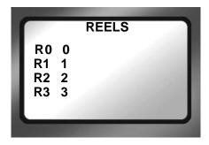
When a disk is formatted, the FS-4Pro HD creates 10 folders, numbered 0-9, on the disk. During recording or playback of a clip, it is possible to place it into folders or play it from up to 10 different reels.
