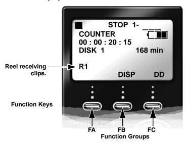
Function settings are user-assignable and available in the Functions screen. Changing a setting with a Function button has the same effect as manually changing the setting.
