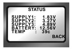
The FS-4 HD Status screen provides details of the systems power state as well as internal temperature. This screen may assist Focus Enhancements Technical Support in determining power and thermal problems with your unit.
