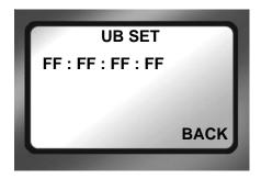
The User Bit Set function provides the ability to change the user bits in the timecode recorded in the video files.
