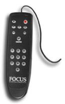
When using the optional wired remote control, use the button pad numbered 0-9 to mark the clips. Any additional button presses during a recording or playback, changes the selected REEL. Once a session is finished, select **Organize REEL** in **Utilities** screen. The marked clips are placed in the REEL folders in sequential order.
