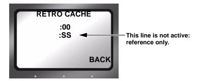
The Retro Cache mode insures that important material at the very start of a recording session is captured. Retro Cache stores in the on board memory a continuous loop of video captured by video camera during pauses. Pressing Record ● begins active recording at the last frame stored in the cache. The resulting video clip has the cached video at the beginning.
