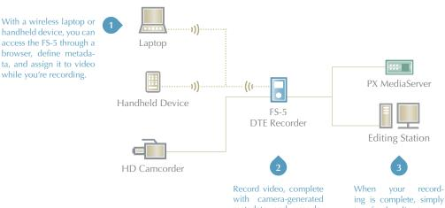
with camera-generated metadata and user-defined metadata received through a wireless connection (optional 802.11 dongle required). When your recording is complete, simply transfer the clips to your media server or editing station—no file conversion is required. Clips are ready to edit instantly.
